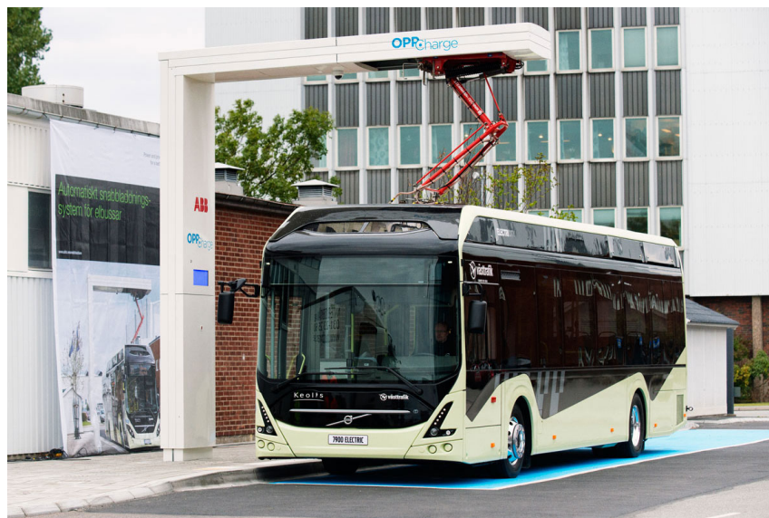
Figure 3: Opportunity ‘flash’ charging pantograph ( Source: OppCharge, n.d. )
