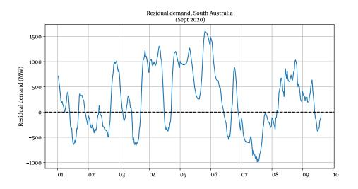
Figure 3: Illustrative residual load in a jurisdiction with high levels of renewable energy generation. The residual load represents the difference between the system demand and power provided by renewable energy generation. Negative regions indicate renewable supply is excess of local demand. This represents the supply that needs to be delivered by other resources to ensure that demand is met.
