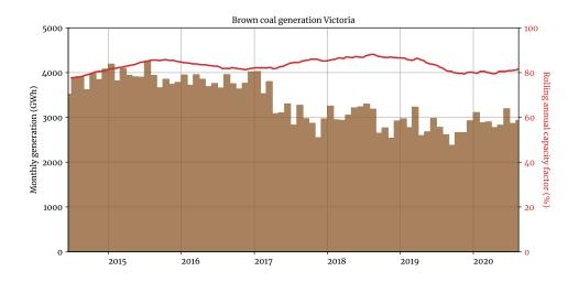
Figure 2: Monthly output of brown coal generators in Victoria since the beginning of financial year 2014. The closure of the Hazelwood power station in early 2017 resulted in improved fleet-wide capacity factor. This fleet-wide capacity factor has since deteriorated and is expected to continue declining, as more renewable energy capacity enters the system.
