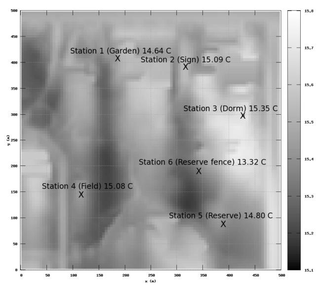
Figure 16—Temperature (in °C) results for ENVI-met model run with observational site data points, 8 April 2011 6:00 am.
