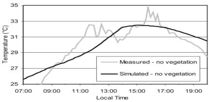
Figure 6–Comparison between measured and simulated air temperature for the existing street canyon (Spangenberg et al. 2008, p. 10)
