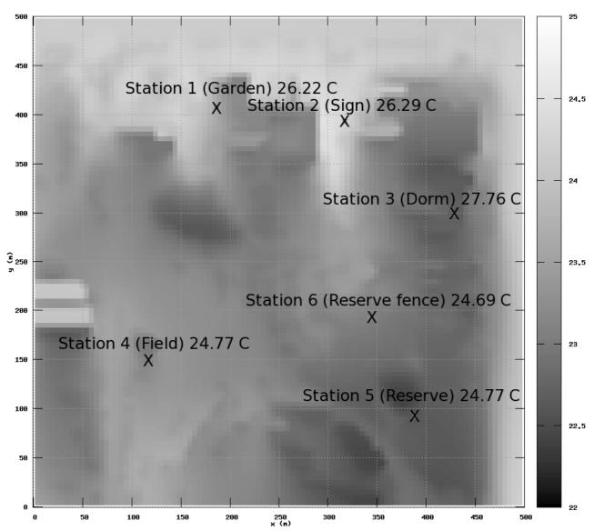
Figure 17–Temperature (in °C) results for ENVI-met model run with observational site data points, 8 April 2011 2:00 pm.
