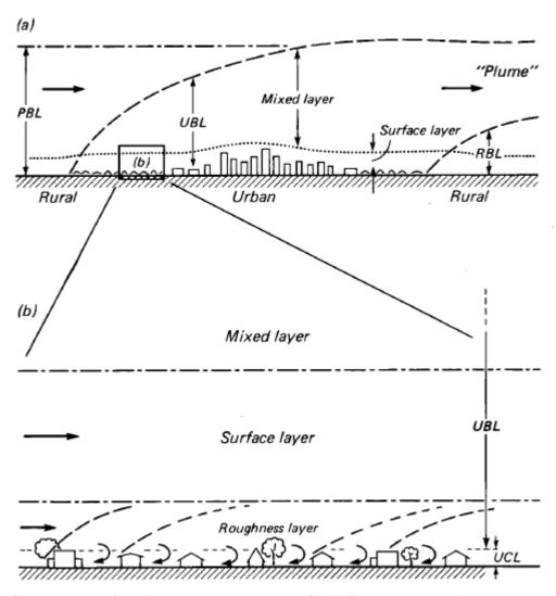
Figure 5–Boundary layer structures over a city (Oke 1988, p. 474)
